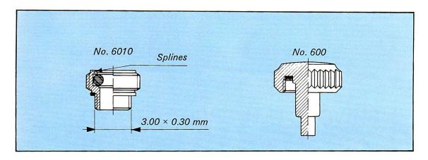
The tube No. 6010 is fitted with a silver washer No. 06020.
